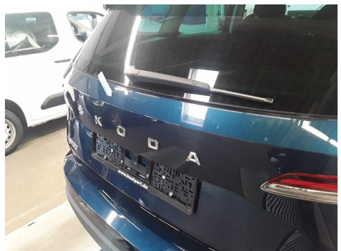
Damage 1: Boot lid / rear door: Boot lid - Dent / paintcoat damage - Smart repair
