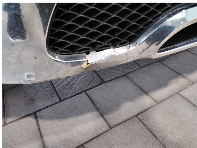
Damage 8: Front bumper: Spoiler - Broken / torn - Replace
