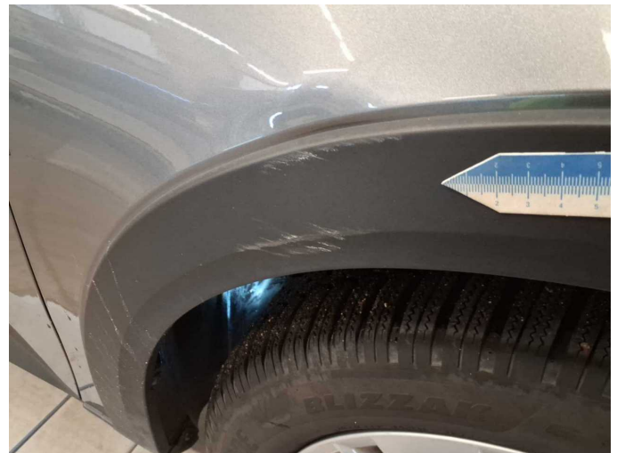
Damage 7: Mudguard - right side: Wheel arch - Scratch(es) - Replace
