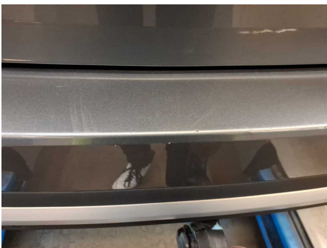
Damage 5: Rear bumper: Rear bumper (Ladekante) - Scratch(es) - Smart repair
