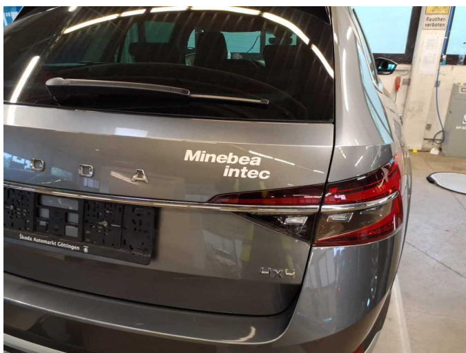
Damage 3: Boot lid / rear door: Boot lid - Glued / labelled - De-glue / neutralise
