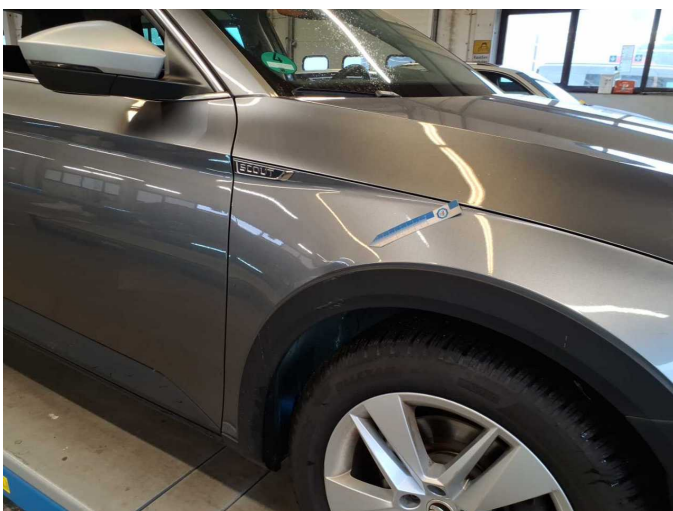
Damage 8: Mudguard - right side: Mudguard - right side - Deformed - Repair and paint
