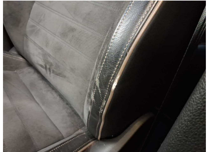
Damage 6: Seat - front: Backrest cover - left side - Scratch(es) - Smart repair
