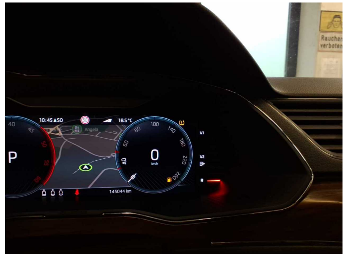
Damage 2: Instrument panel: Indicator light (Rdks) - on - Perform diagnosis
