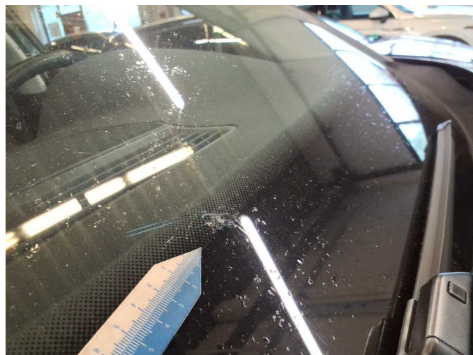
Damage 9: Vehicle glazing: Windscreen - Broken / torn - Replace
