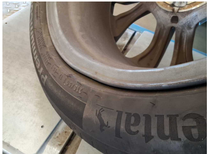
Damage 5: 2nd wheel set: 1 alloy rim - Deformed - Replace
