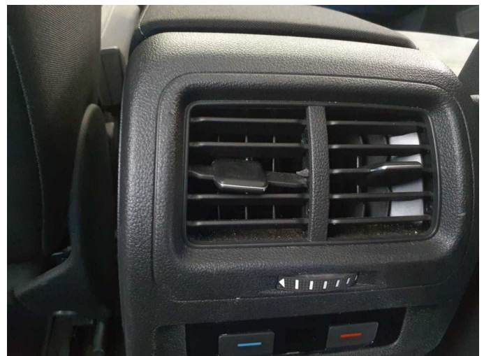
Damage 5: Instrument panel: Air nozzle - centre (Hinten) - Broken / torn - Replace
