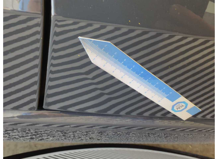
Damage 6: Door - front right side: Door - Deformed - Paint
