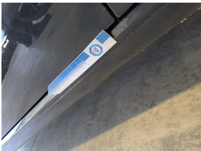
Damage 7: Sill - right side: Sill - Deformed - Repair and paint
