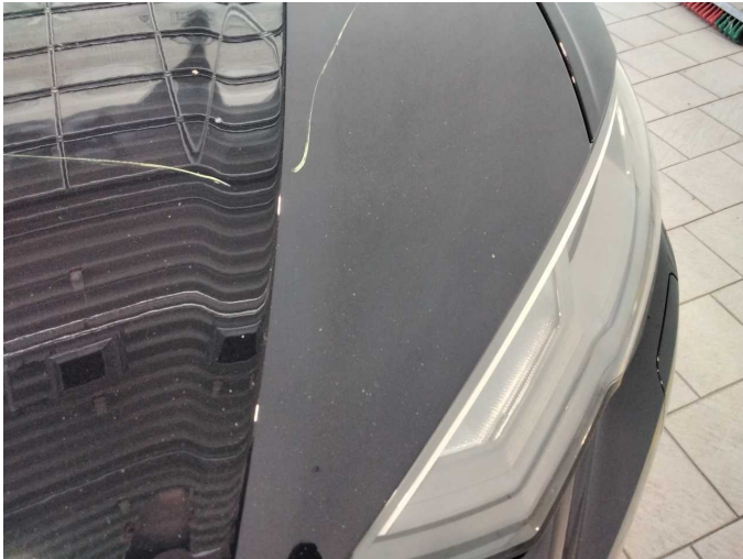
Damage 5: Bonnet: Bonnet - Stone chips - Paint
