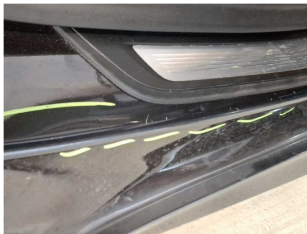
Damage #12: Side panel - rear right side: Sill - Scratched - Smart repair
