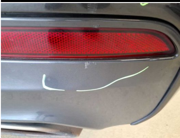
Damage #5: Rear bumper: Spoiler - Scratched - Loss in value
