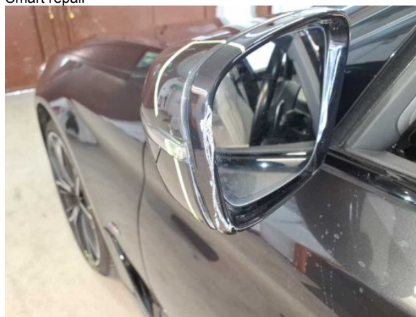
Damage #14: Wing mirror - left side: Mirror housing - Damag... - Replace
