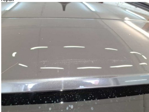
Damage #13: Boot lid / rear door: Rear spoiler - Scratched - Smart repair
