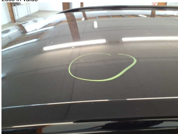
Damage #4: Roof: Roof - dent(s) - Smooth repair work
