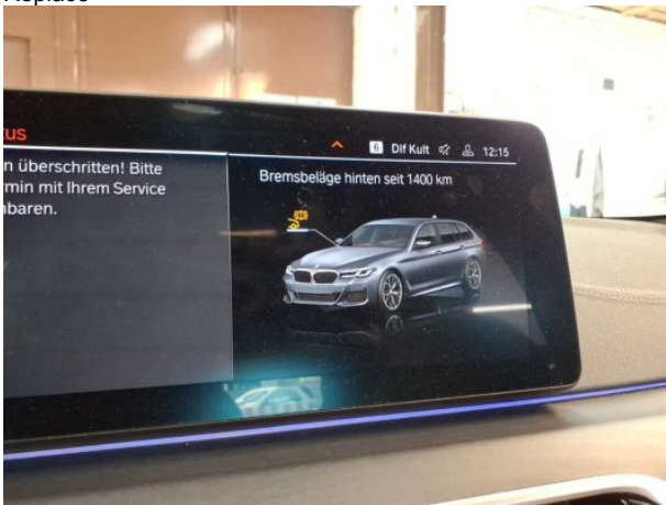
Damage #15: Braking system: Brake discs and pads - rear - Due - Replace
