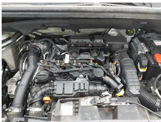
Missing part 1: Engine: Engine cover - Missing - Replace
