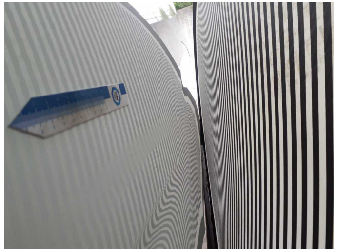
Damage 7: Side panel - rear left side: Side panel - Dent / paintcoat damage - Paint
