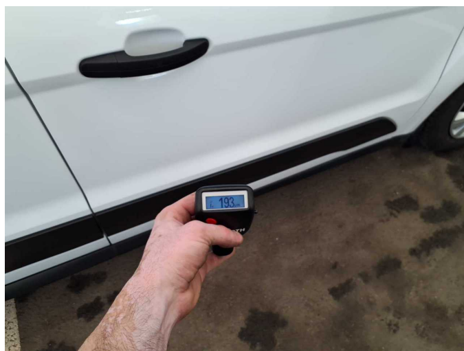
Repainting 4: Door - front right side
