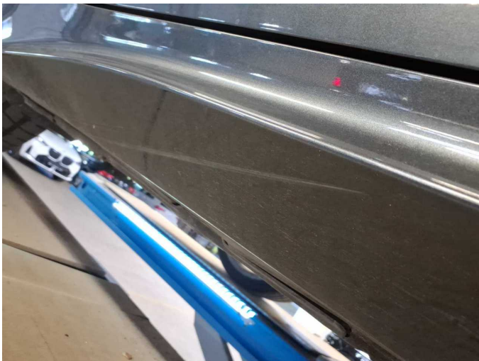
Damage 3: Sill - right side: Trim - Scratched - Paint
