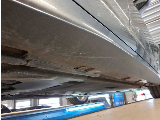
Damage 3: Sill - right side: Trim - Scratched - Paint
