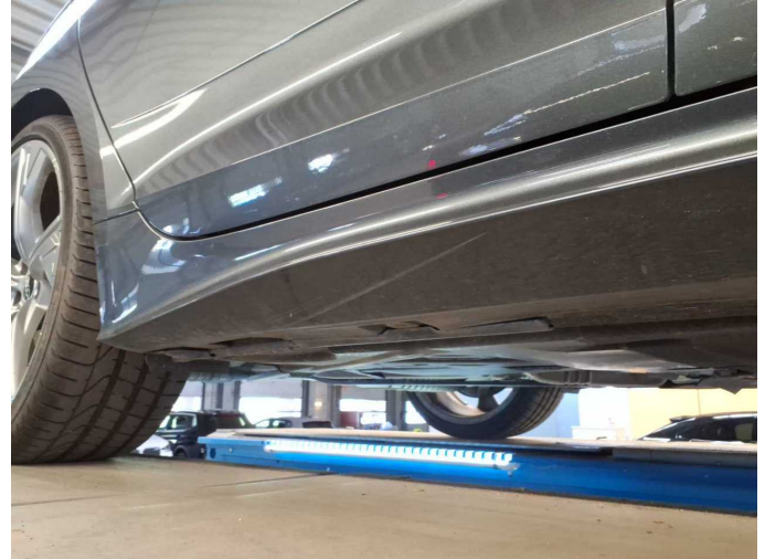
Damage 3: Sill - right side: Trim - Scratched - Paint
