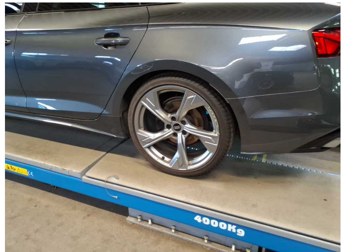
Damage 4: Wheel / tyres: Alloy rim - rear left side (Materialabtrag) - Scratched - Loss in value
