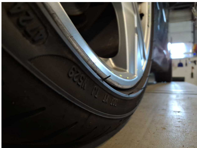
Damage 5: Wheel / tyres: Alloy rim - rear right side (Materialabtrag) - Scratched - Loss in value
