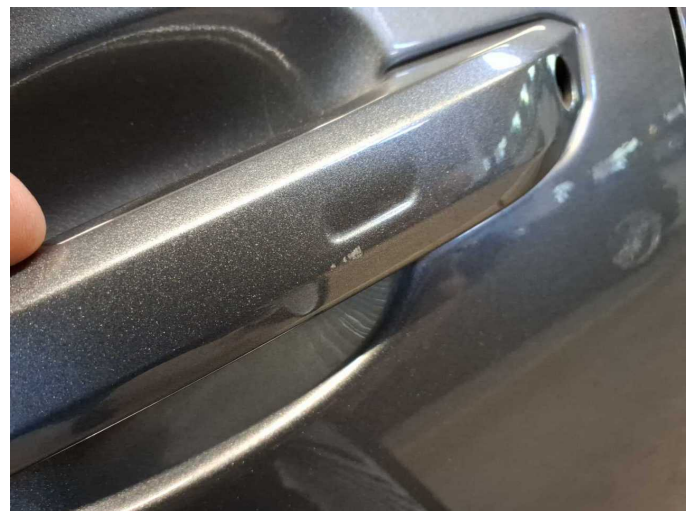
Wear and tear 5: Door - front left side: Door handle - outside - Scratch(es) - Smart repair
