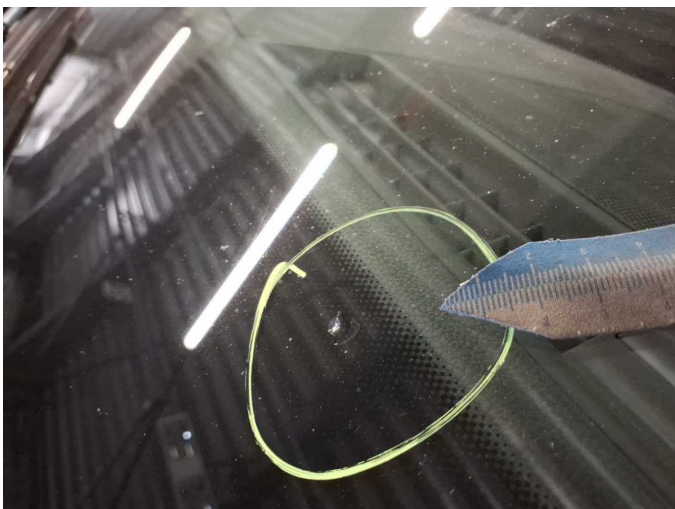
Damage 11: Vehicle glazing: Windscreen (Rissbildung) - Stone chips - repair according to calculation
