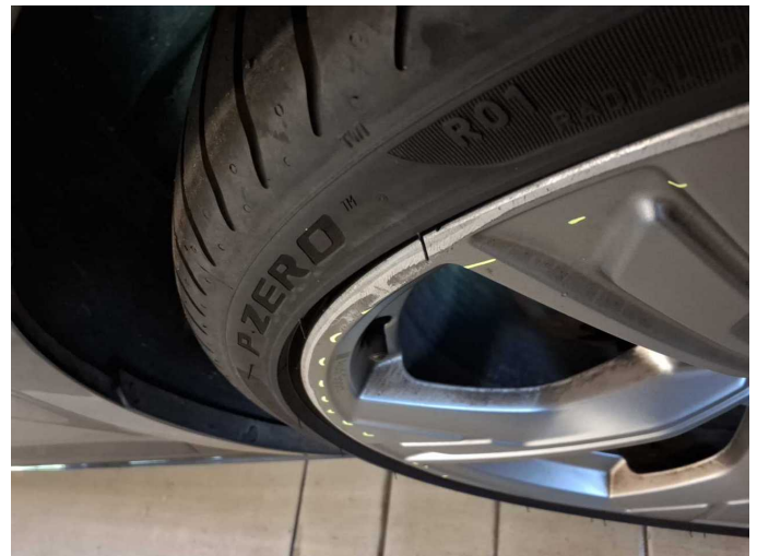
Damage 7: Wheel / tyres: Alloy rim - front right side (Materialabtrag) - Scratched - Loss in value
