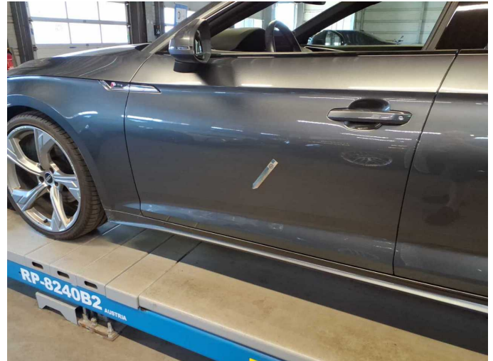
Damage 8: Door - front left side: Door (Einschlüsse) - Unprofessionally repaired - Repair and paint
