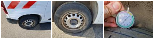
Tyre FR, Out of tolerance, Replace
