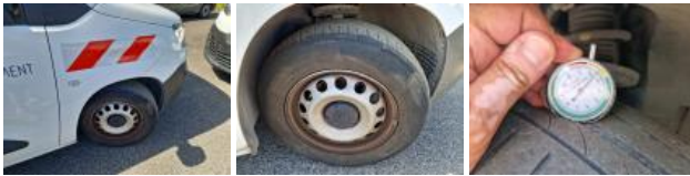
Tyre FL, Out of tolerance, Acceptable
