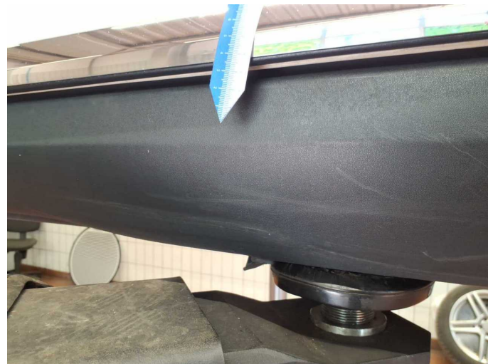
Wear and tear 2: Sill - left side: Trim - Scratch(es) - No deduction
