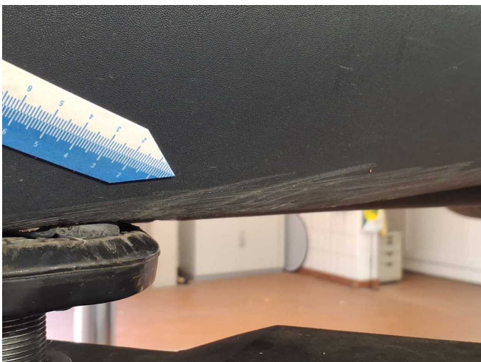
Damage 7: Sill - right side: Trim - Scratch(es) - Replace
