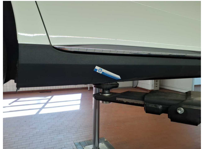
Damage 7: Sill - right side: Trim - Scratch(es) - Replace
