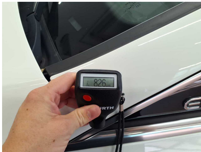
Repainting 6: Roof rail - left side
