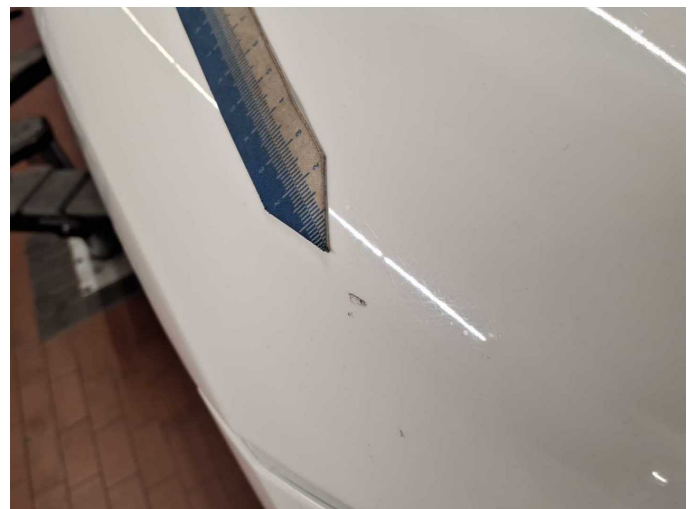
Damage 10: Bonnet: Bonnet - Stone chips - Paint
