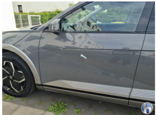
4. Tür Vorne - Links Kratzer - Smart Repair
