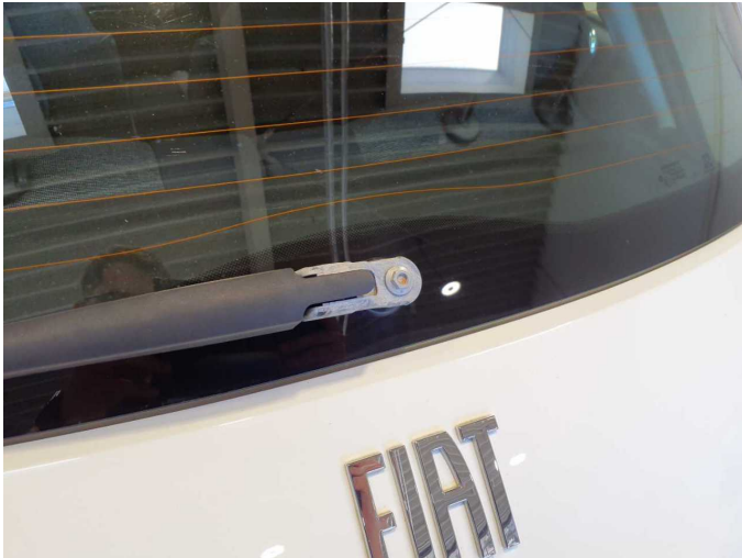
Damage 4: Screen cleaning: Wiper arm - rear - Missing - Replace
