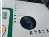
Windscreen, Stone chip(s), Windscreen repair
