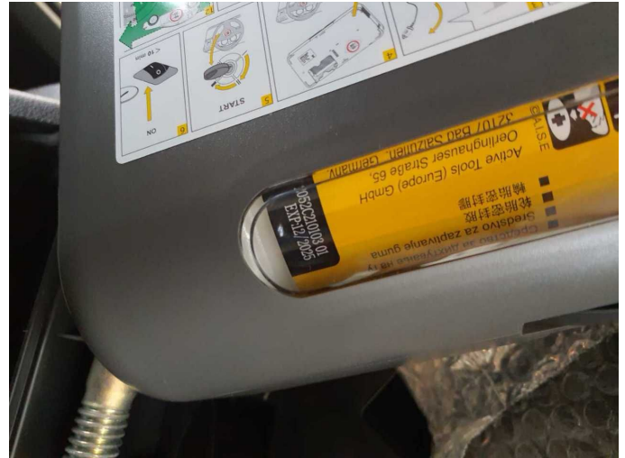
Damage 1: Equipment: Tirefit filler - Expired - Replace
