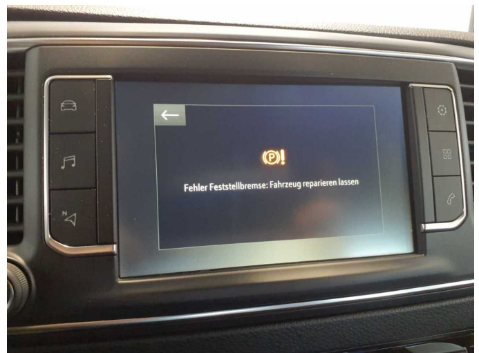
Damage 3: Braking system: Parking brake / hand brake (Feststellbremse) - Functional / admissibility - Perform diagnosis
