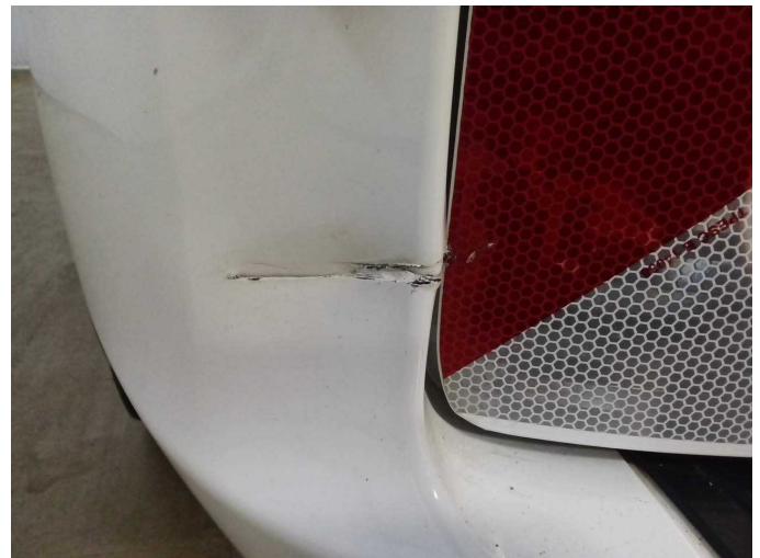
Damage 4: Rear bumper: Bumper - rear left side - Scratched - Repair and paint
