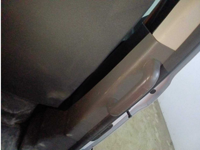
Wear and tear 4: Trim / covers: B-pillar - trim - interior, right side - Scratch(es) - No deduction
