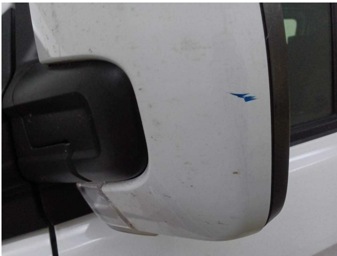
Wear and tear 2: Wing mirror - left side: Mirror housing - Scratch(es) - No deduction
