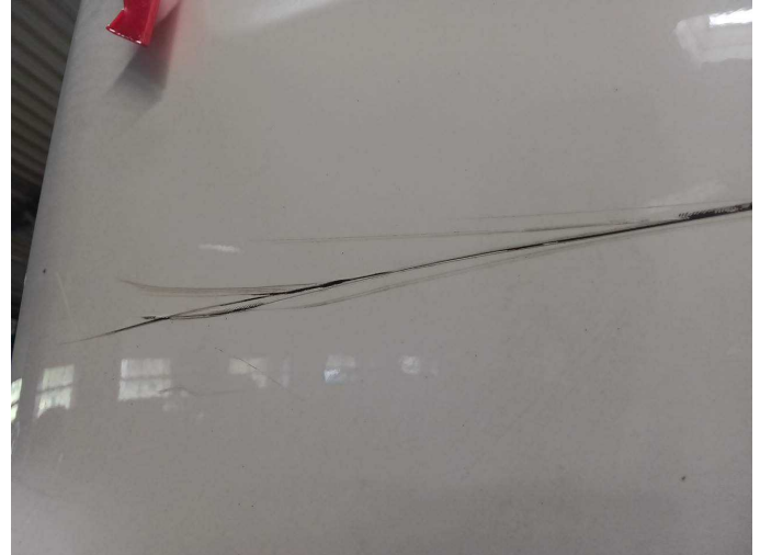
Damage 3: Rear bumper: Bumper - rear right side - Scratched - Paint
