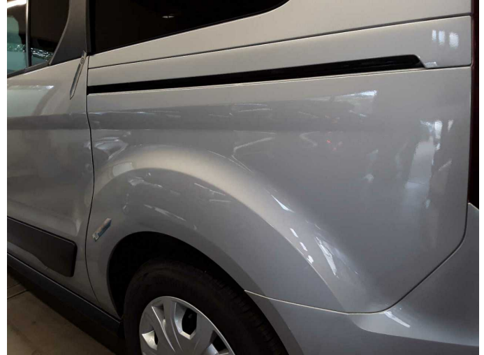
Damage 7: Side panel - rear left side: Side panel - Deformed - Repair and paint
