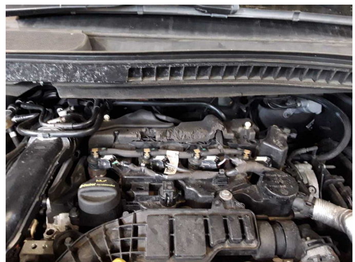
Damage 3: Engine: Engine cover - Damaged - Replace
