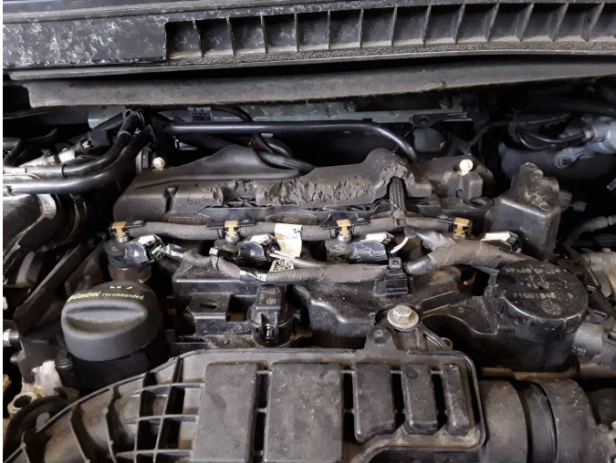
Damage 3: Engine: Engine cover - Damaged - Replace
