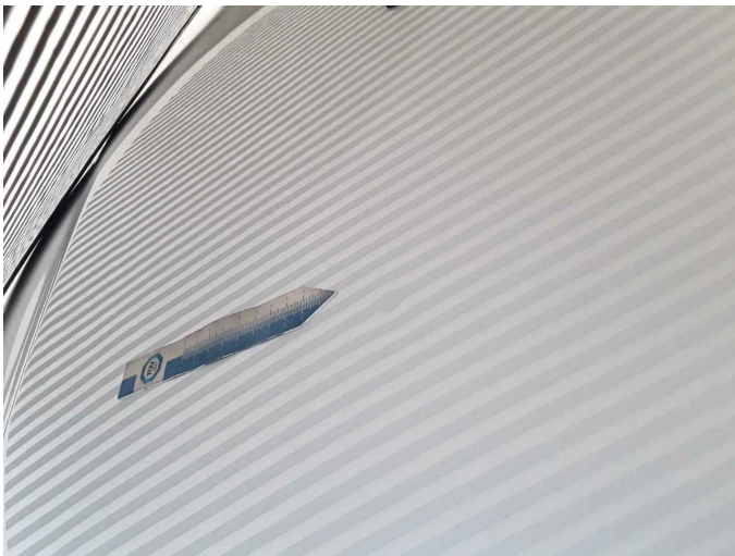
Damage 4: Bonnet: Bonnet - dent(s) - Smooth repair work
