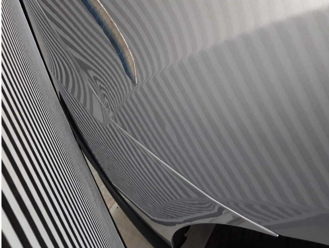
Damage 6: Side panel - rear right side: Side panel - Deformed - Repair and paint
