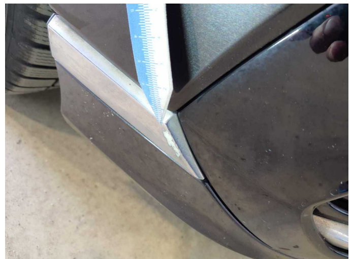
Damage 1: Trim / covers: Trim / covers - Scratch(es) - Loss in value
