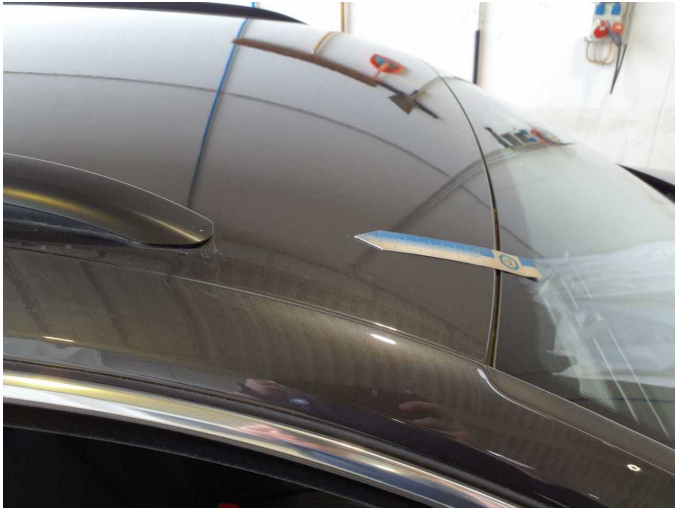
Damage 10: Roof: Roof - Corrosion - Repair and paint
