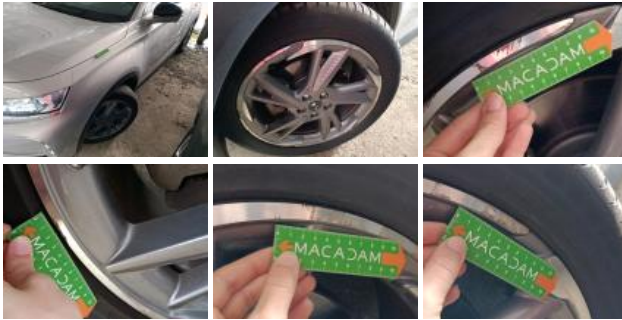
Tyre RL, Out of tolerance, Replace
