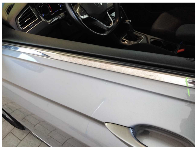
Damage 4: Door - front left side: Strip - outer - Paint defect - Replace
