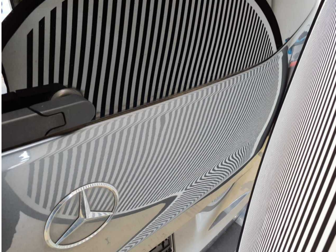
Wear and tear 8: Boot lid / rear door: Boot lid - Dent / paintcoat damage - No deduction
