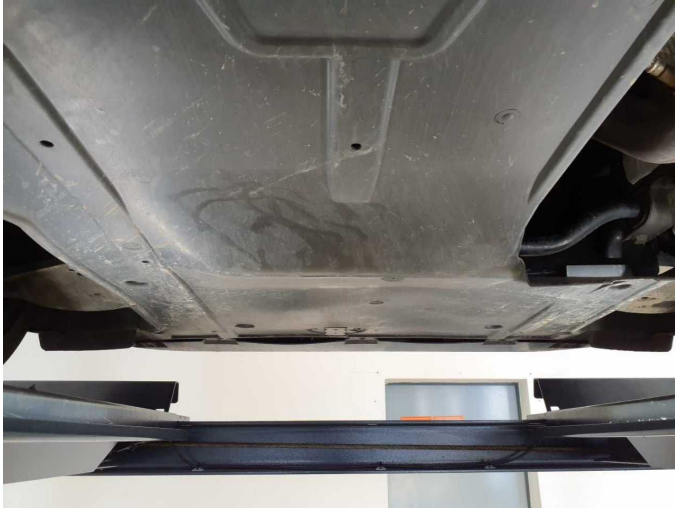
Damage 3: Body: Underbody panelling - Broken / torn - Replace
