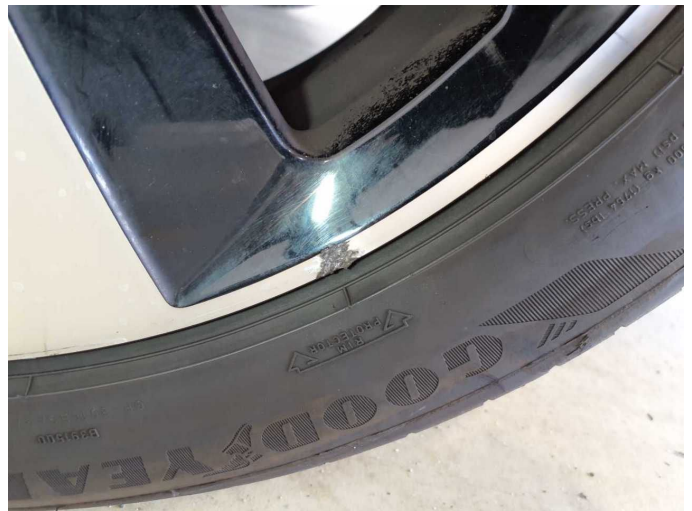
Wear and tear 9: Wheel / tyres: Alloy rim - rear left side - Scratch(es) - No deduction
