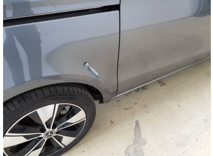
Damage 4: Side panel - rear right side: Side panel (Einschlüsse-Mehrkosten möglich) - Unprofessionally repaired - Conditioning
