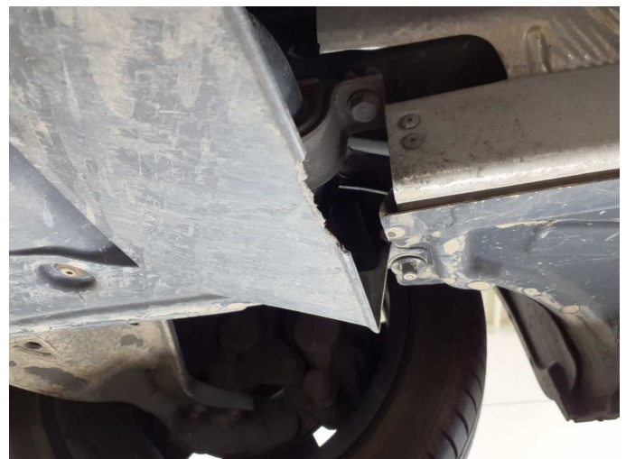
Damage 3: Body: Underbody panelling - Broken / torn - Replace
