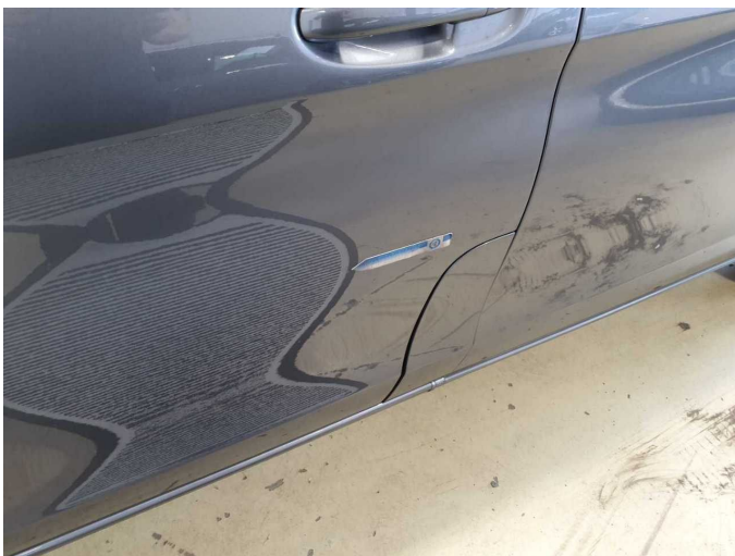
Damage 5: Door - front left side: Door (Lack Druckstelle) - Unprofessionally repaired - Smart repair
