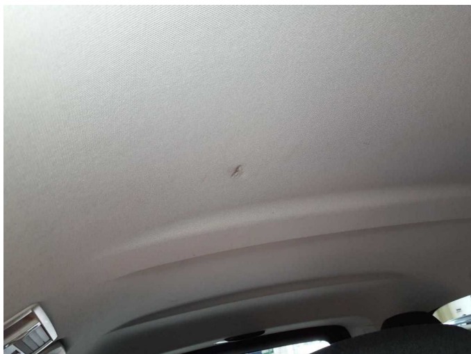
Damage 8: Trim / covers: Roof lining - Broken / torn - Replace
