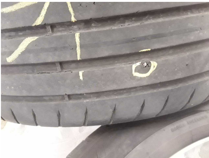
Damage 3: 2nd wheel set: 1 tyre - Damaged - Replace
