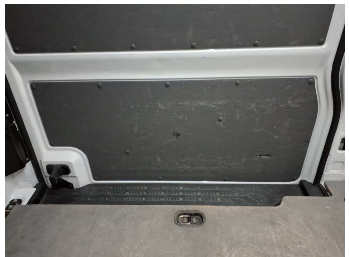
Damage 2: Sliding door, right: Trim (Unten) - Broken / torn - Replace
