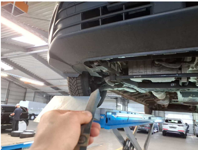
Damage 4: Drive train: Sleeve prop shaft - front left side (+ Rechts) - Broken / torn - Replace
