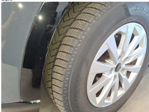
Damage #2: Mudguard - left side: Wheel well extension - Scratch(es) - Smart repair
