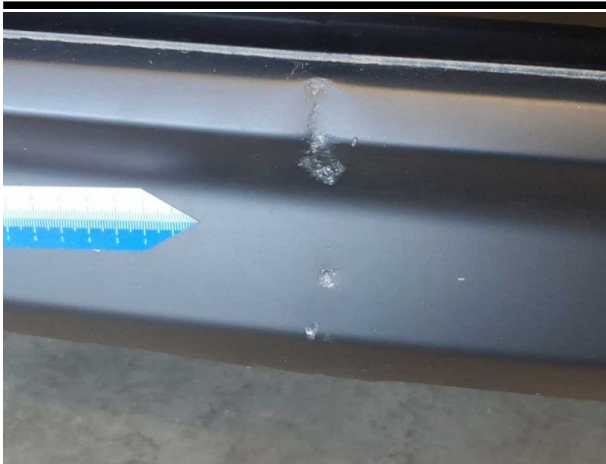
Damage #5: Rear bumper: Spoiler - Deformed - Replace
