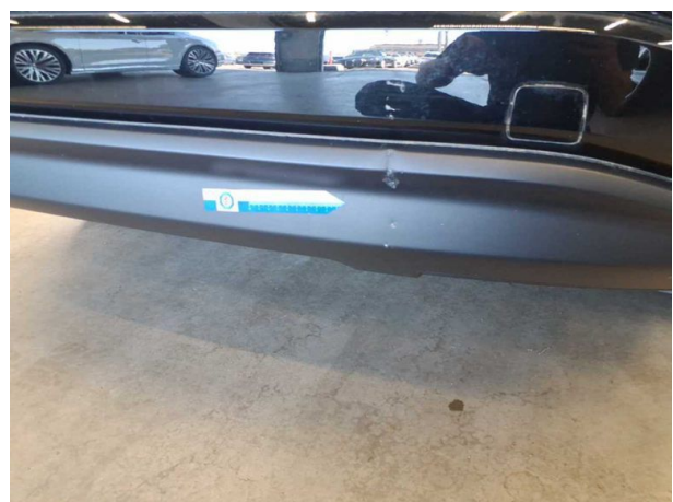
Damage #5: Rear bumper: Spoiler - Deformed - Replace
