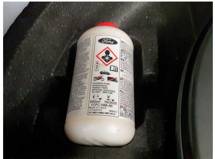
Damage 1: Equipment: Tirefit filler - Expired - Replace
