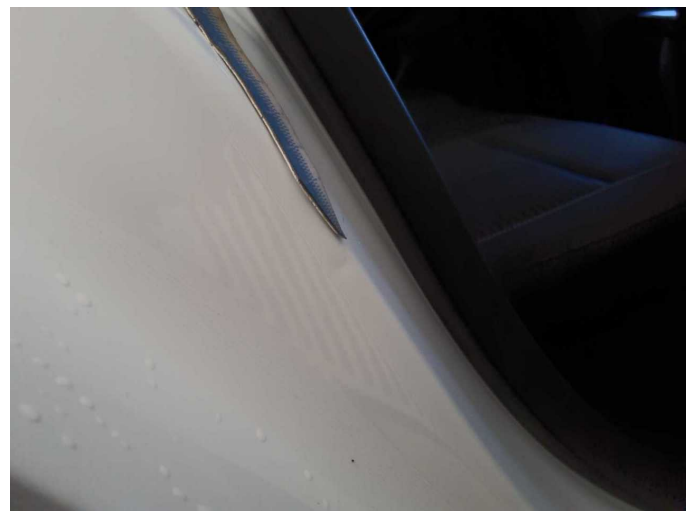
Damage 2: Side panel - rear right side: Sill - dent(s) - Smart repair
