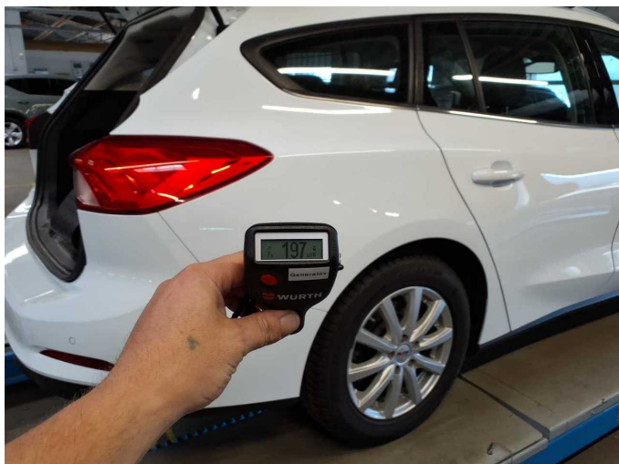
Repainting 1: Side panel - rear right side
