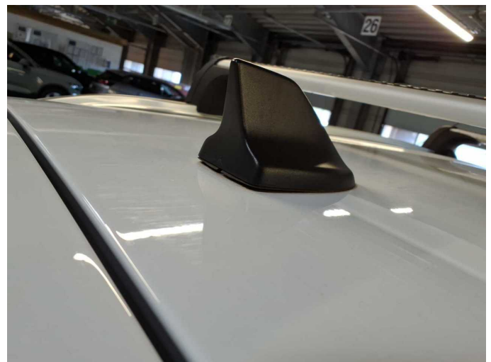
Damage 8: Roof: Aerial - Loose - Un- / install
