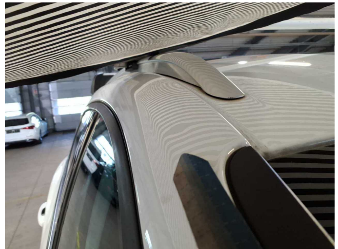
Damage 7: Roof: Roof rail - right side - dent(s) - Smooth repair work
