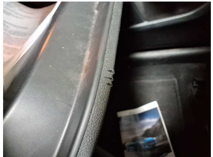
Damage 13: Instrument panel: Glove box - Scratched - Replace
