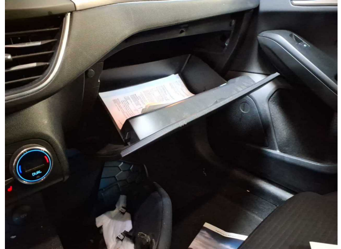
Damage 13: Instrument panel: Glove box - Scratched - Replace
