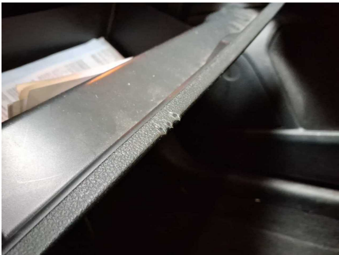
Damage 13: Instrument panel: Glove box - Scratched - Replace
