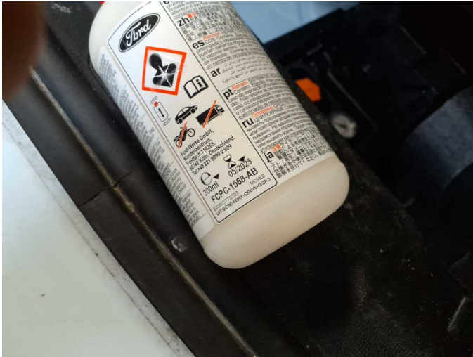
Damage 3: Equipment: Tirefit filler - Expired - Replace
