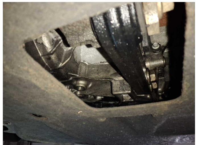
Damage 4: Gearbox: Gearbox - Leaking - Perform diagnosis
