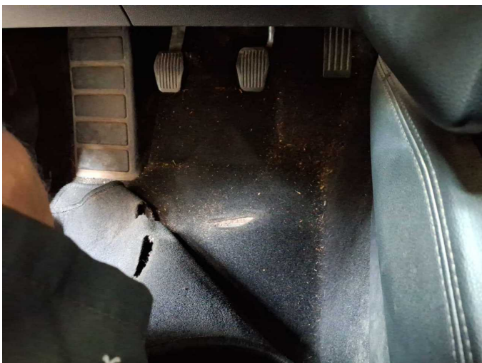
Damage 14: Trim / covers: Floor covering - front left side - Broken / torn - Replace
