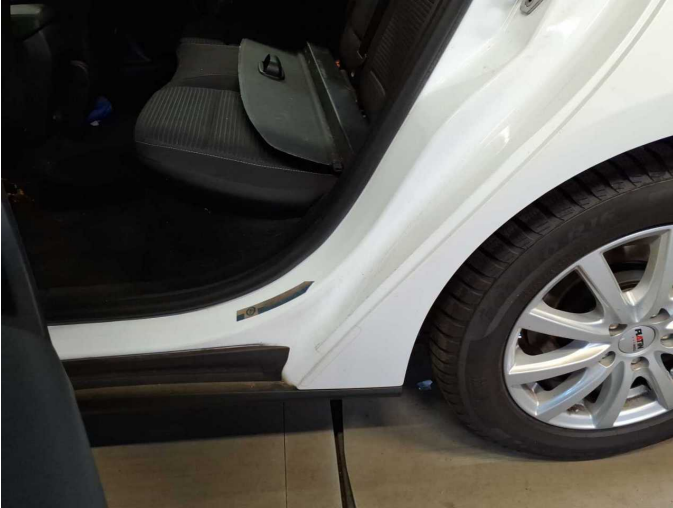
Damage 9: Side panel - rear left side: Sill - Dent / paintcoat damage - Smart repair
