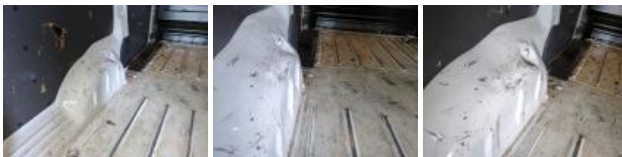
Wheel aperture RR, Dent(s) and scratch(es), Repair and paint (complete)
