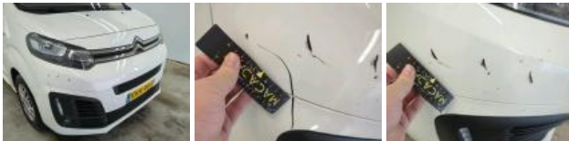
Bumper F, Scratch(es), Repair and paint (complete)
