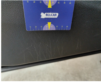
Front Left Door Interior Coating // Replace Completely-scratch
