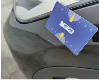
Door Rear Left // Smart Repair Small-scratch
