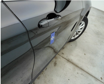
Rocker Panel Left // Smart Repair Medium-scratch + dent
