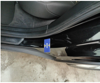
Rocker Panel Left // Smart Repair Medium-scratch + dent
