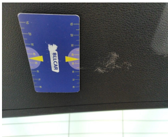
Trunk Lid Interior Coating / Complete Panel / Replace-scratch
