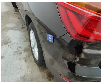
Rear Bonnet // Repair & Painting-scratch + dent
