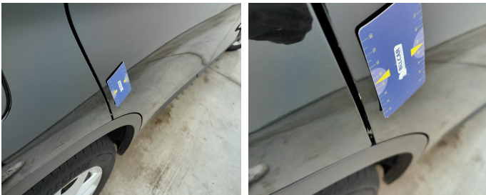
Door Rear Right // Smart Repair Small-scratch
