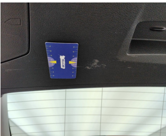
Trunk Lid Interior Coating / Complete Panel / Replace-scratch
