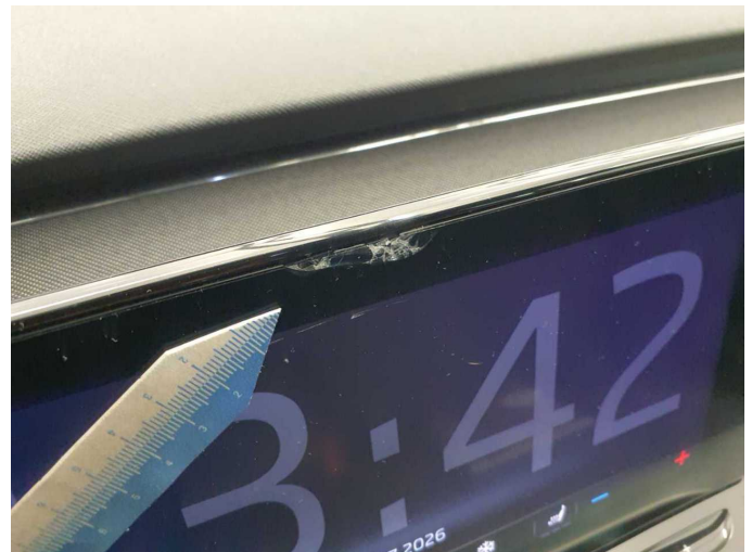
Damage 9: Multimedia system: Navigation system - Damaged - Replace
