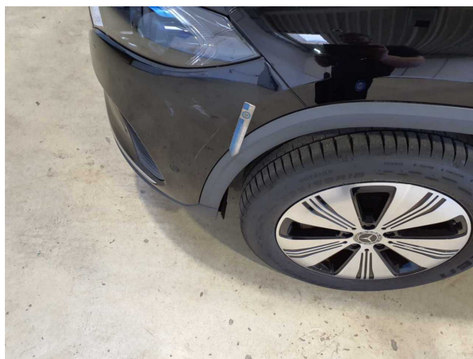
Damage 10: Mudguard - left side: Wheel well extension - Scratch(es) - Replace
