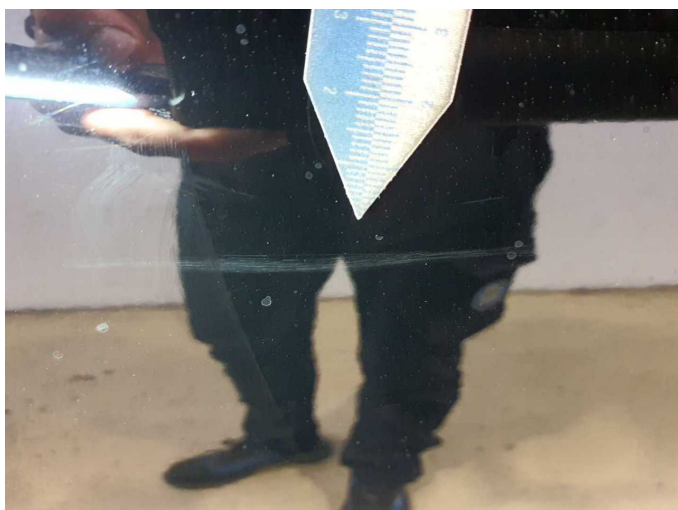
Damage 8: Door - front right side: Door - Scratch(es) - Smart repair
