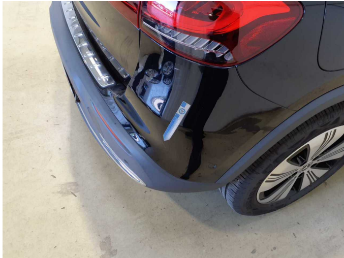
Damage 15: Rear bumper: Bumper - rear right side - Scratch(es) - Paint
