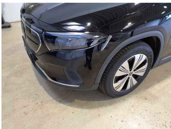
Damage 14: Front bumper: Front bumper - Dent / paintcoat damage - Repair and paint
