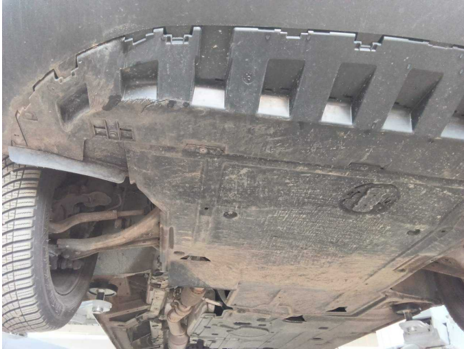
Damage 5: Body: Underbody panelling - Broken / torn - Replace
