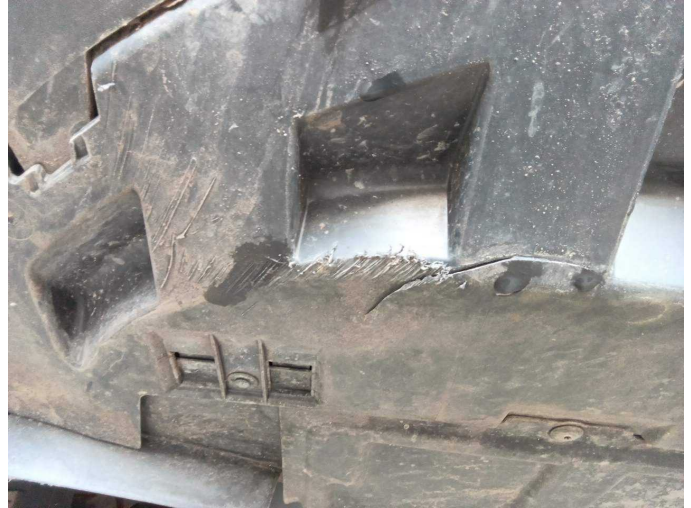
Damage 5: Body: Underbody panelling - Broken / torn - Replace
