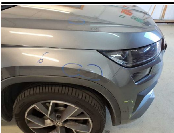
Damage #12: Mudguard - right side: Mudguard - right side - Dent / paintcoat damage - Repair and paint
