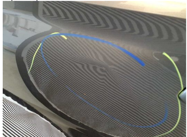
Damage #18: Door - front left side: Door - Dent / paintcoat damage - Replace
