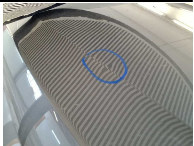
Damage #17: Bonnet: Bonnet - Dent / paintcoat damage - Repair and paint
