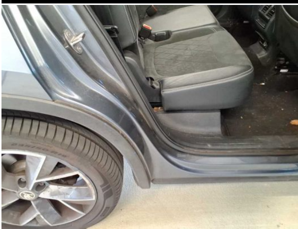
Damage #5: Side panel - rear right side: Sill - Dent / paintcoat damage - Smart repair
