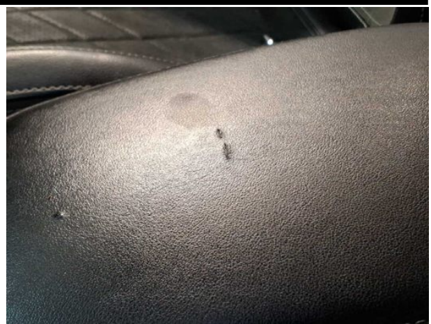
Damage #9: Seat - front: armrests - Damaged - Replace
