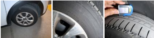
Wheel cover FR, Deformed / Strained, Replace
