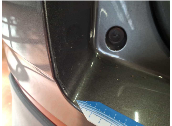
Damage 13: Rear bumper: Rear bumper - Scratch(es) - Paint
