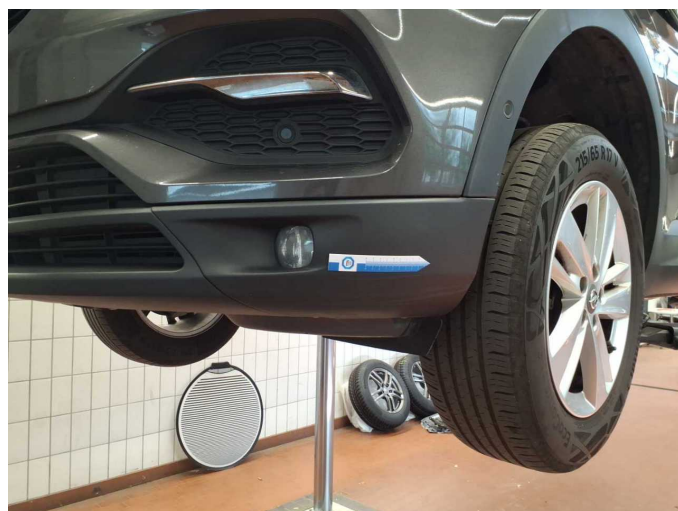
Damage 3: Front bumper: Front bumper (unpainted) - Scratched - Replace
