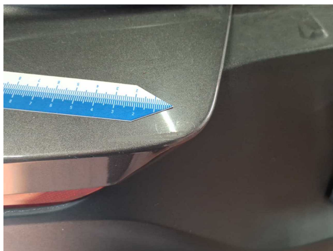
Damage 13: Rear bumper: Rear bumper - Scratch(es) - Paint
