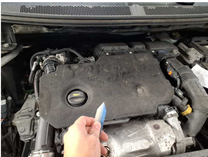
Wear and tear 2: Engine: Engine cover - Damage caused by marten / rodent - No deduction
