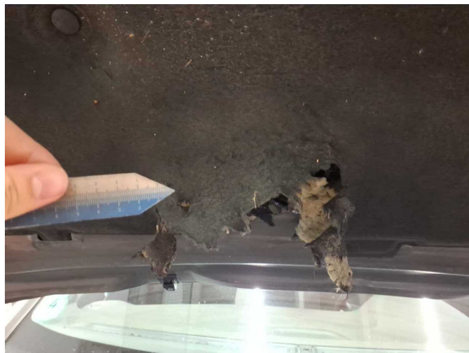
Damage 12: Bonnet: Insulation lining - Damage caused by marten / rodent - Replace
