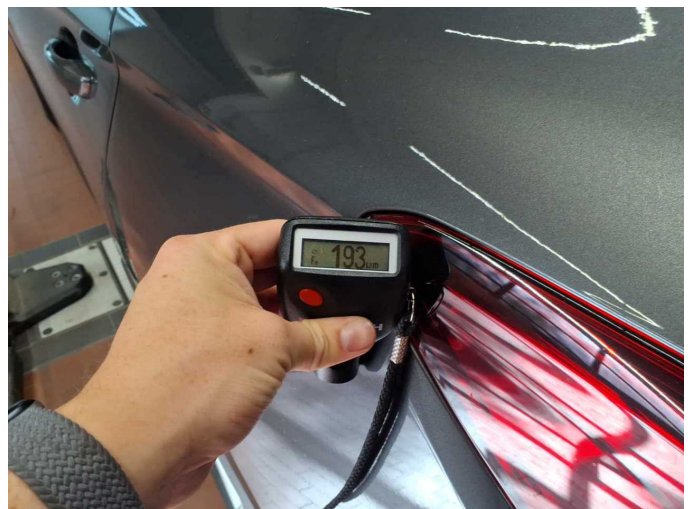
Repainting 1: Side panel - rear left side
