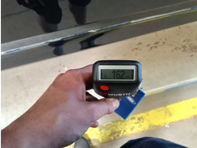
Repainting 1: Door - front right side
