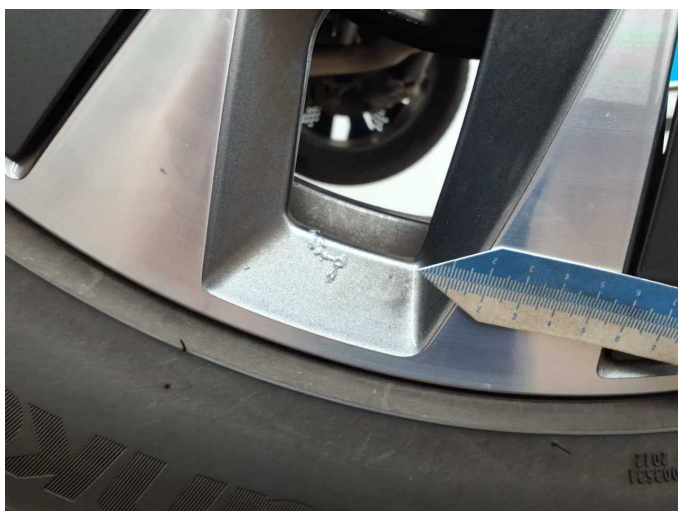
Damage 4: Wheel / tyres: Alloy rim - rear left side - Corrosion - Loss in value
