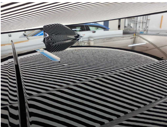
Damage 3: Roof: Roof - dent(s) - Smooth repair work
