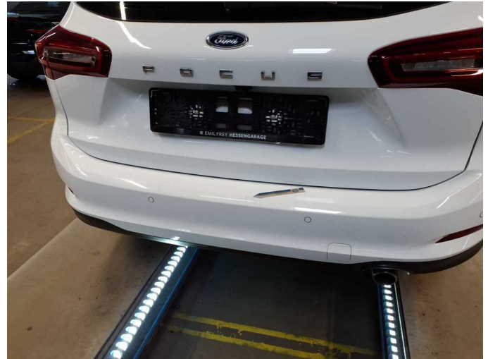
Damage 6: Rear bumper: Rear bumper - Scratched - Paint
