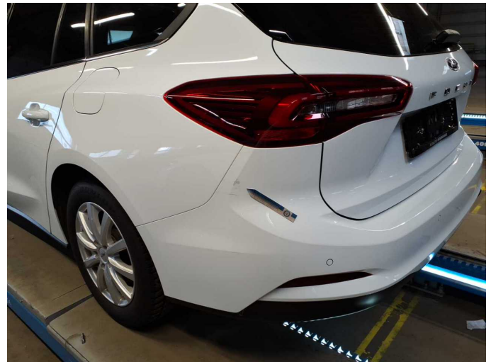
Damage 6: Rear bumper: Rear bumper - Scratched - Paint
