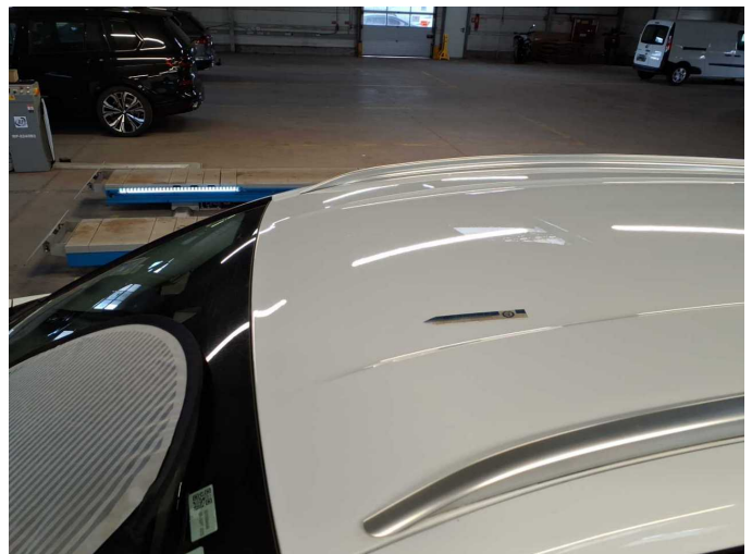
Damage 1: Roof: Roof - dent(s) - Smooth repair work
