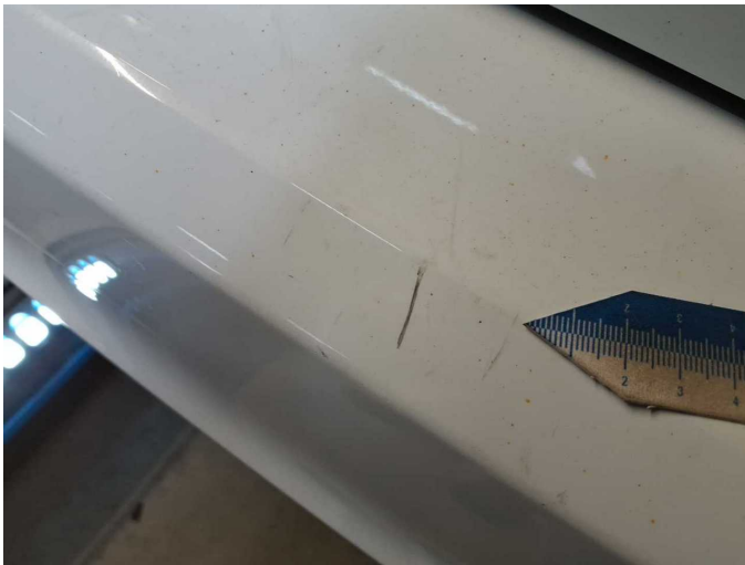
Damage 6: Rear bumper: Rear bumper - Scratched - Paint
