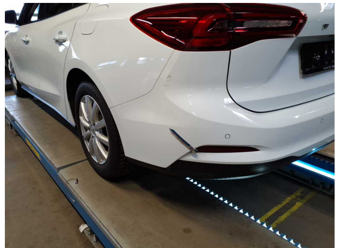
Damage 6: Rear bumper: Rear bumper - Scratched - Paint
