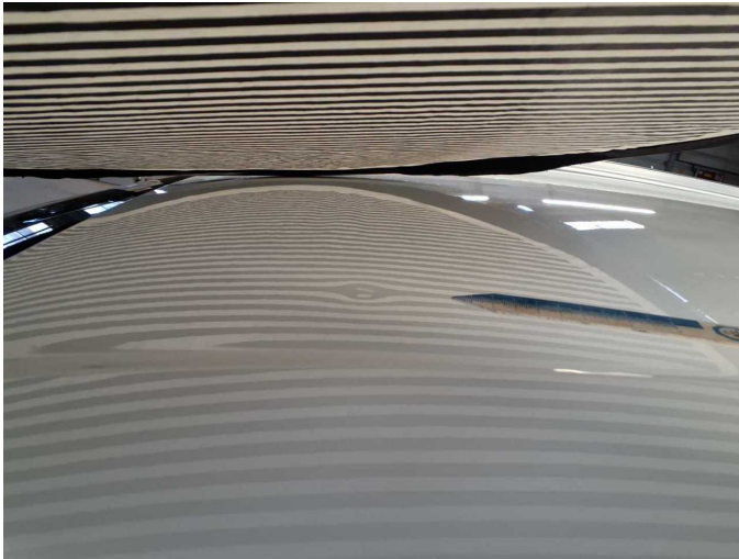
Damage 1: Roof: Roof - dent(s) - Smooth repair work
