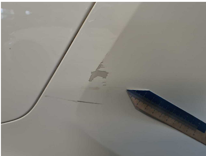
Damage 6: Rear bumper: Rear bumper - Scratched - Paint
