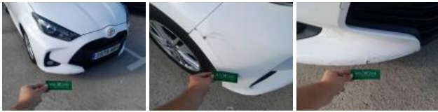
Bumper F, Scratch(es), Repair and paint (complete)
