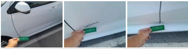
Door RL, Scratch(es), Repair and paint (complete)
