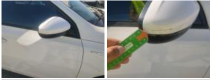
Outside rear-view mirror R, complete, Scratch(es), Repair and paint (complete)
