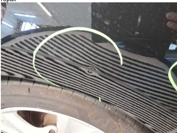
Damage #9: Side panel - rear right side: Side panel - Dent / paintcoat damage - Repair and paint
