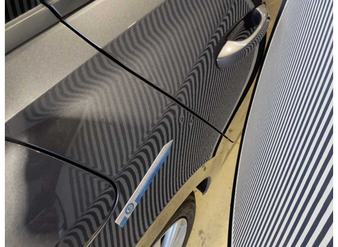
Damage 7: Side panel - rear right side: Side panel - Dent / paintcoat damage - Smart repair
