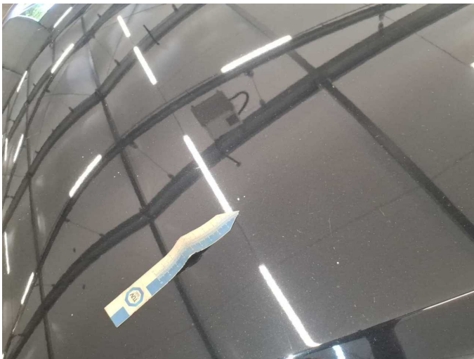
Damage 17: Bonnet: Bonnet - Scratched - Paint
