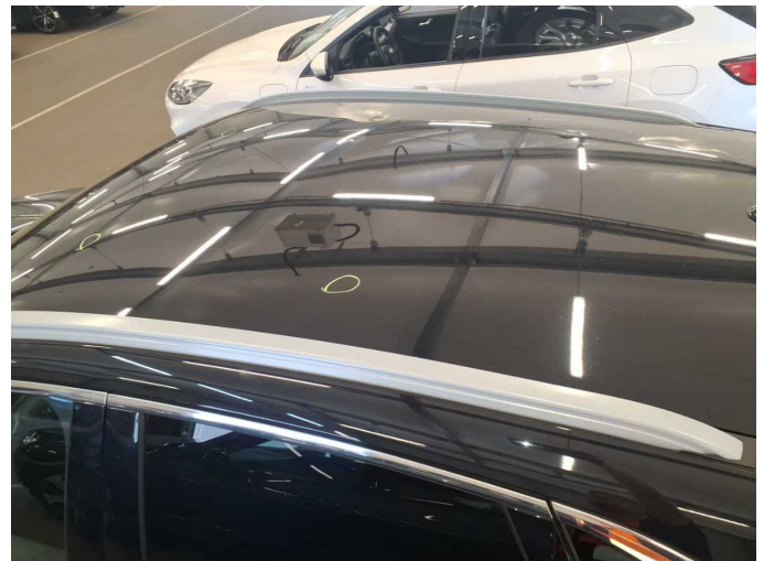
Damage 10: Roof: Roof - dent(s) - Smooth repair work
