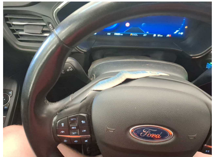
Damage 3: Steering system: Steering wheel (Blende Multifunktionslenkrad) - Paint defect - Loss in value
