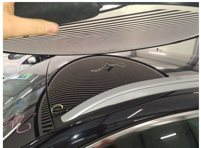
Damage 10: Roof: Roof - dent(s) - Smooth repair work
