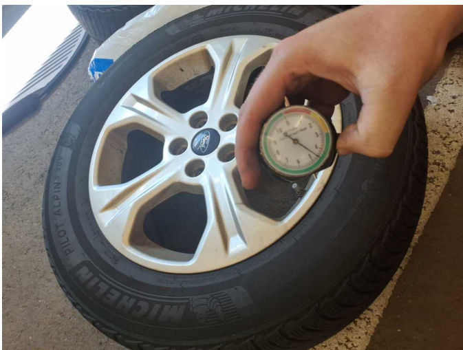
Damage 11: 2nd wheel set: Tyres - complete set - Does not meet the leasing specifications - Replace
