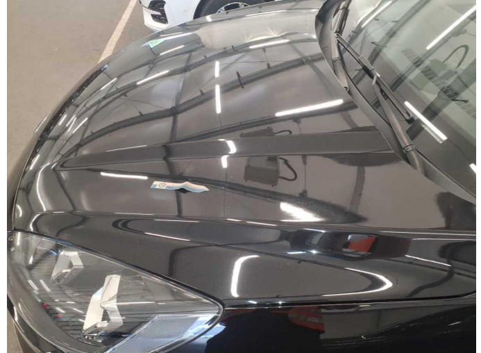
Damage 17: Bonnet: Bonnet - Scratched - Paint
