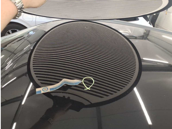
Damage 10: Roof: Roof - dent(s) - Smooth repair work
