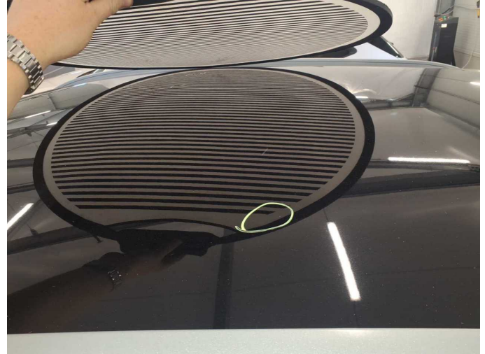
Damage 10: Roof: Roof - dent(s) - Smooth repair work
