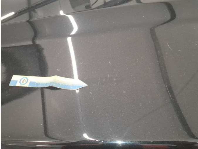
Damage 17: Bonnet: Bonnet - Scratched - Paint
