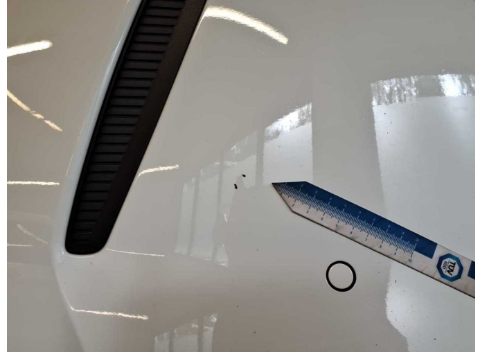
Damage 6: Front bumper: Front bumper - Scratch(es) - Paint
