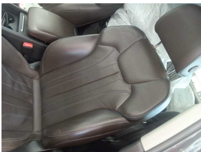
Damage 5: Seat - front: Backrest - left side - Worn - Smart repair
