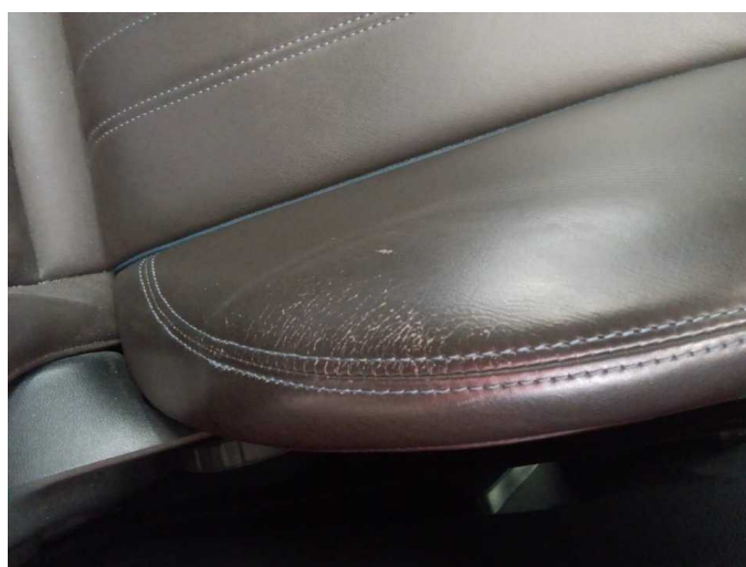
Damage 5: Seat - front: Backrest - left side - Worn - Smart repair
