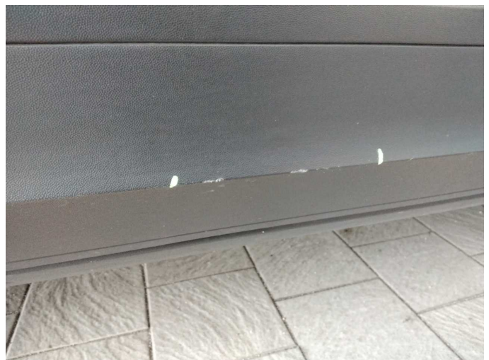
Damage 4: Door - front right side: Brightware - lower - Scratch(es) - Loss in value
