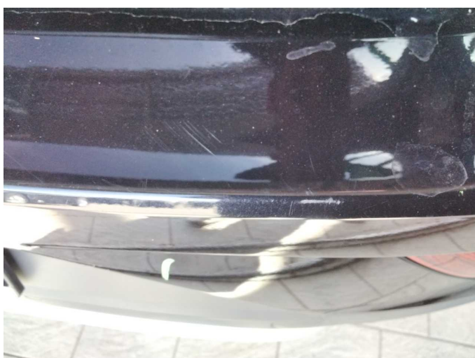
Damage 15: Rear bumper: Rear bumper - Scratch(es) - Paint
