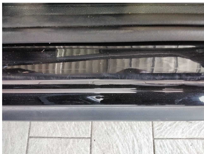
Damage 10: Sill - left side: Sill - Scratch(es) - Smart repair
