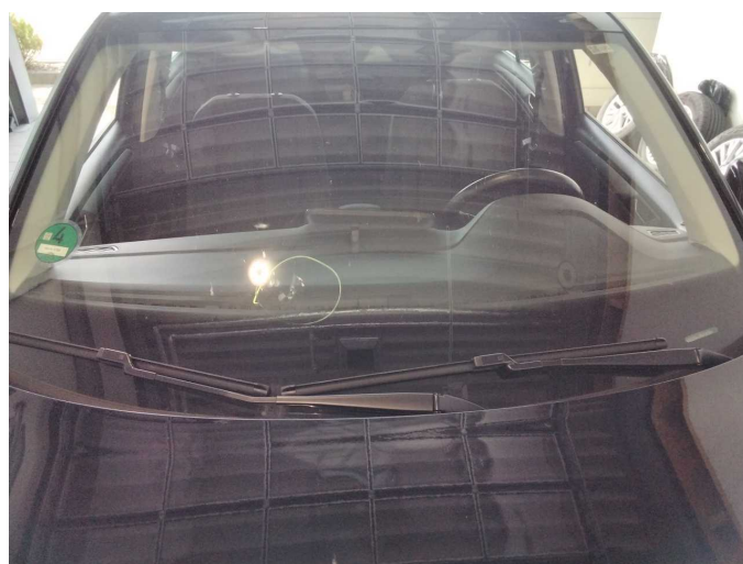
Damage 16: Vehicle glazing: Windscreen - Broken / torn - Replace
