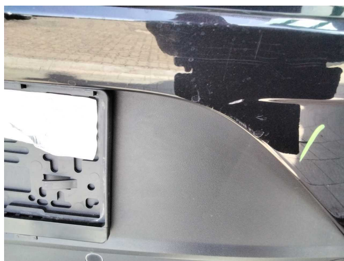
Damage 15: Rear bumper: Rear bumper - Scratch(es) - Paint
