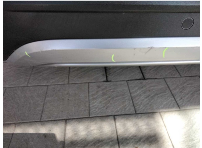
Damage 14: Rear bumper: Spoiler - Scratch(es) - Replace
