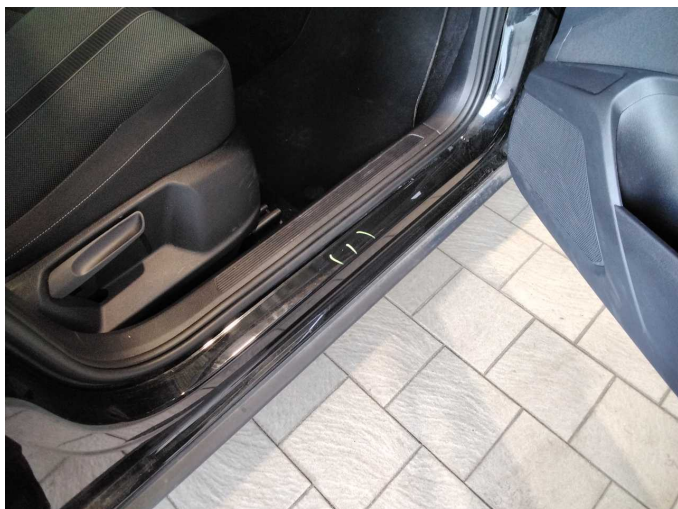
Damage 11: Sill - right side: Sill - Dent / paintcoat damage - Smart repair
