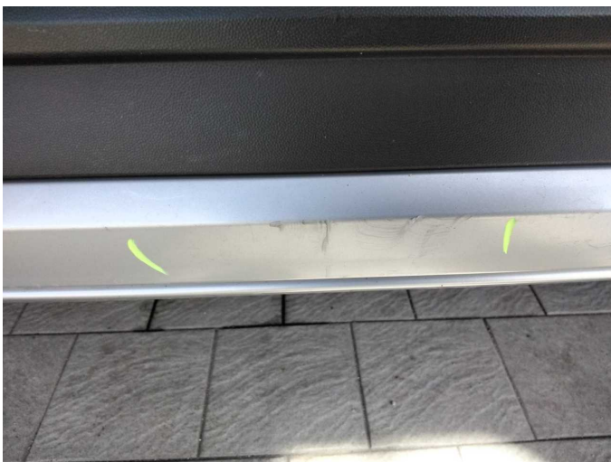
Damage 14: Rear bumper: Spoiler - Scratch(es) - Replace
