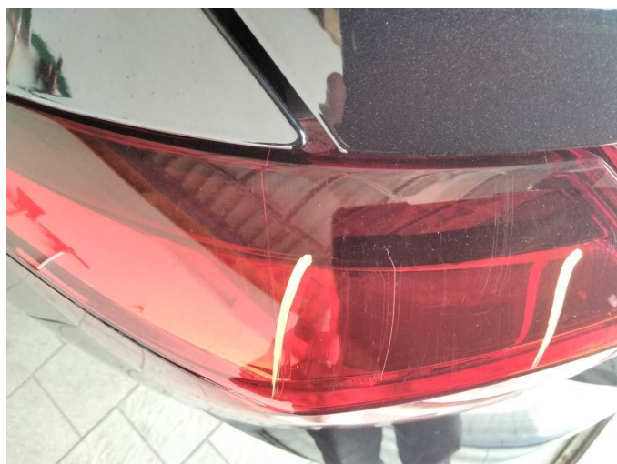
Damage 6: Tail light: Tail lamp - left side - Scratch(es) - Loss in value
