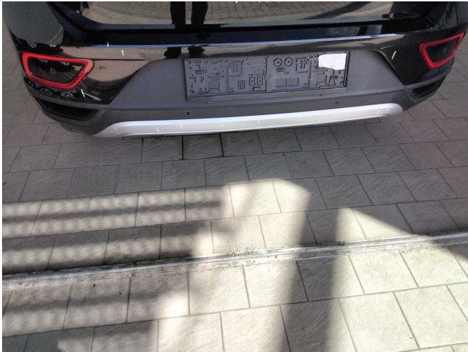
Damage 14: Rear bumper: Spoiler - Scratch(es) - Replace
