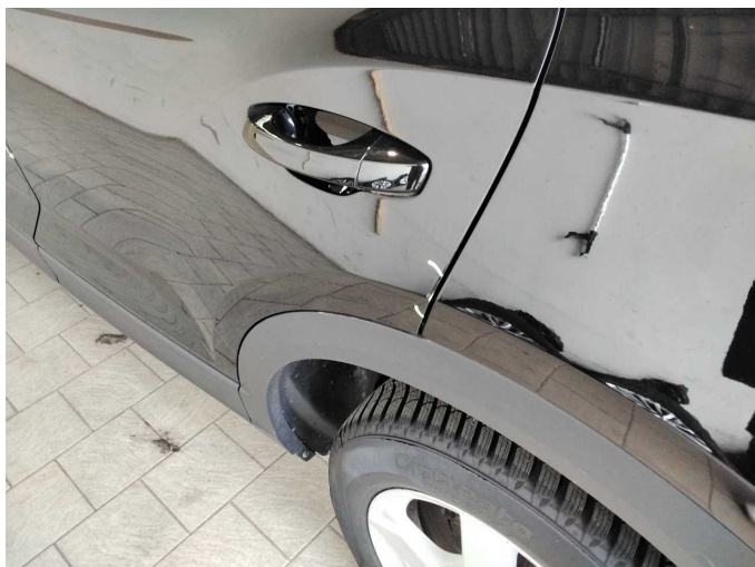
Damage 8: Door - rear left side: Door edge - Scratch(es) - Smart repair
