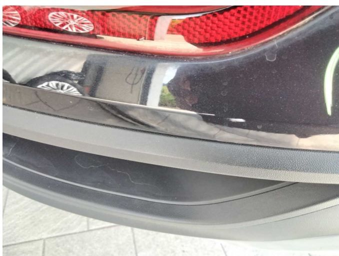
Damage 15: Rear bumper: Rear bumper - Scratch(es) - Paint
