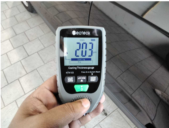
Repainting 1: Door - rear left side
