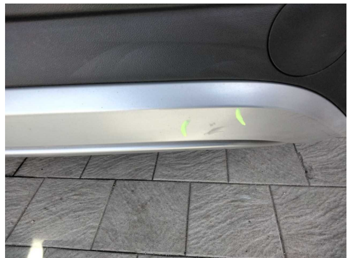
Damage 14: Rear bumper: Spoiler - Scratch(es) - Replace
