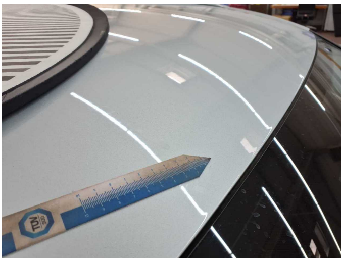
Damage 17: Roof: Roof - Dent / paintcoat damage - Paint
