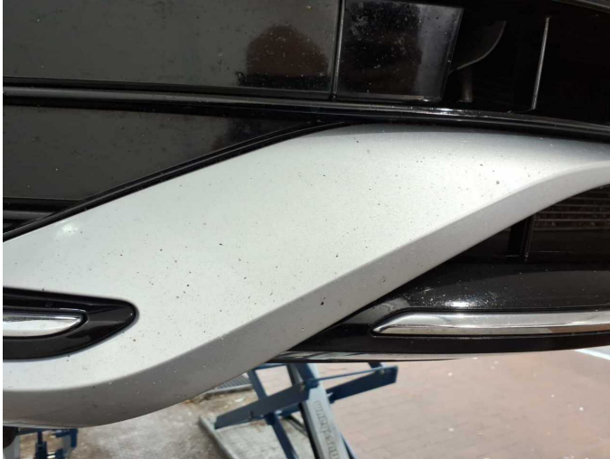
Damage 16: Front bumper: Front bumper - Paint defect - Paint
