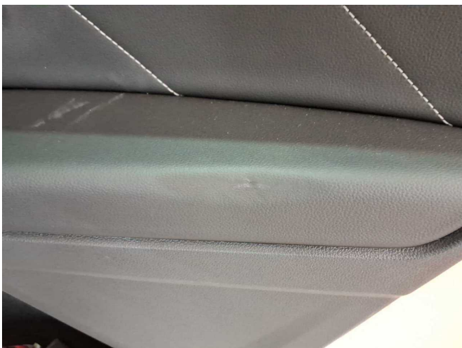
Damage 8: Trim / covers: Door trim - rear right side - Damaged - Loss in value
