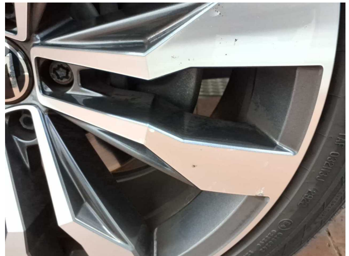
Damage 12: Wheel / tyres: Alloy rim - front right side - Scratch(es) - Replace
