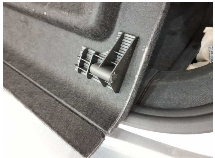
Damage 10: Interior: Rear shelf - Broken / torn - Replace
