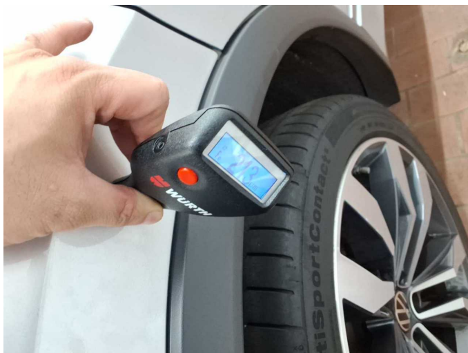
Side panel - rear right side: 213 µm
