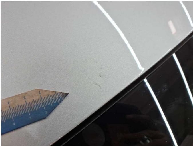
Damage 17: Roof: Roof - Dent / paintcoat damage - Paint
