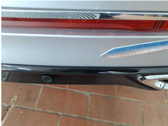
Damage 15: Rear bumper: Rear bumper - Dent / paintcoat damage - Paint
