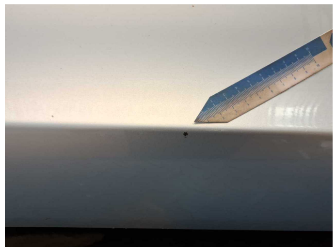
Wear and tear 7: Trim / covers: Door trim - rear right side - Scratched - No deduction
