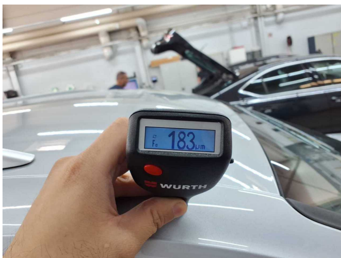
Roof rail - right side: 183 µm
