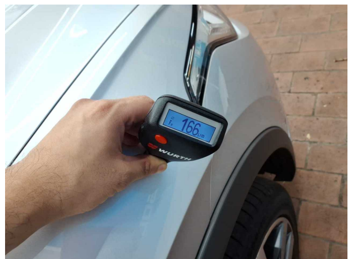
Mudguard - right side: 166 µm
