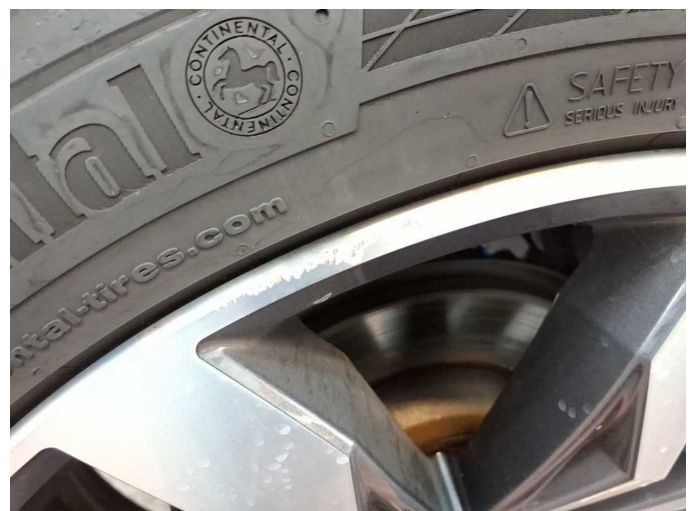
Damage 11: Wheel / tyres: Alloy rim - rear right side - Damaged - Loss in value
