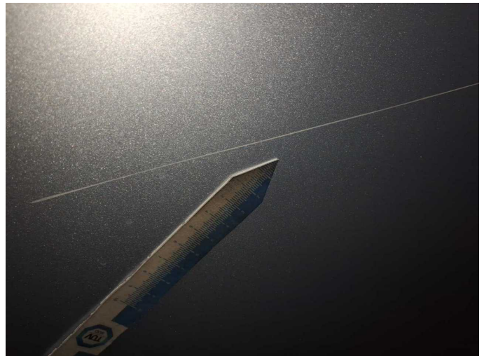
Damage 5: Door - rear right side: Door - Dent / paintcoat damage - Repair and paint
