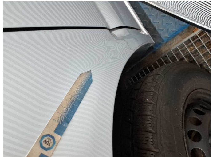
Damage 3: Side panel - rear right side: Side panel - dent(s) - Repair and paint
