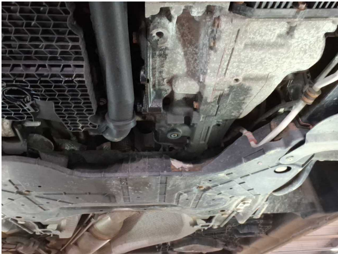
Damage 1: Gearbox: Gearbox - Leaking - Perform diagnosis
